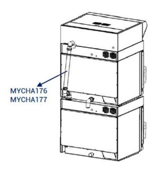
Figure 4. Hood connection in stacked ovens
