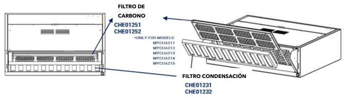
Figure 8. Removal of condensation filter and carbon filter
