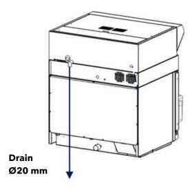
Figure 3. Drain connection
