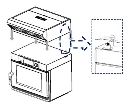
Figure 1. Positioning of the condensation hood
