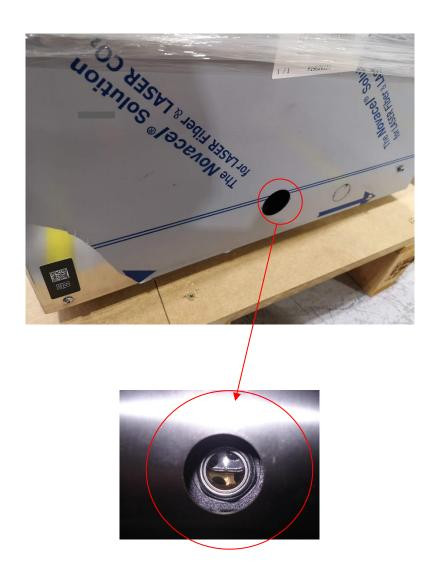
Illustration 1. Rear display for checking the oil level
