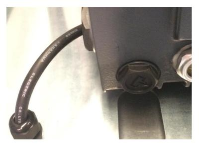
Illustration 5. Remove the oil drainage plug
