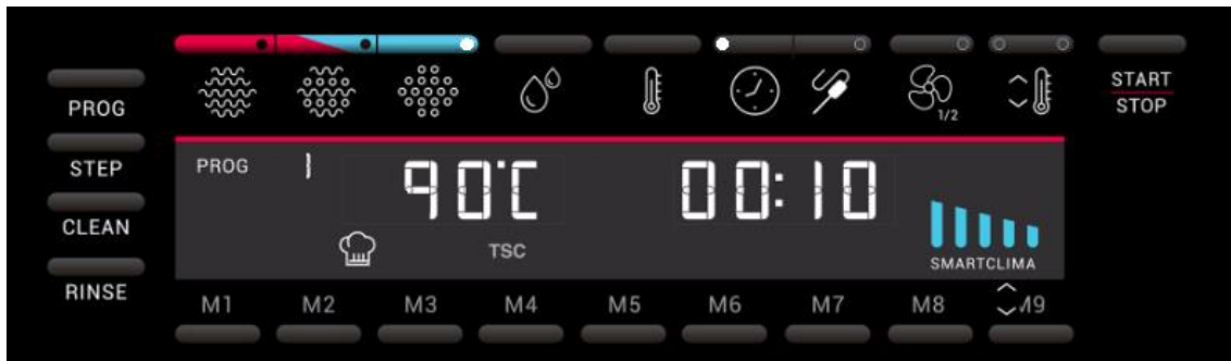
Figure 9. Example. Cooking at 90° in steam for 10 minutes
