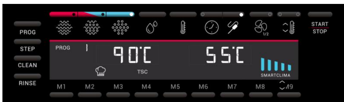
Figure 14. Example. Cooking 90°C in steam mode and core temperature 55°C
