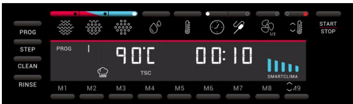
Figure 11. Example. Cooking 90°C in steam mode for 10 minutes
